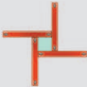
Captive column tie bolts and nuts are permanently attached to each element.
